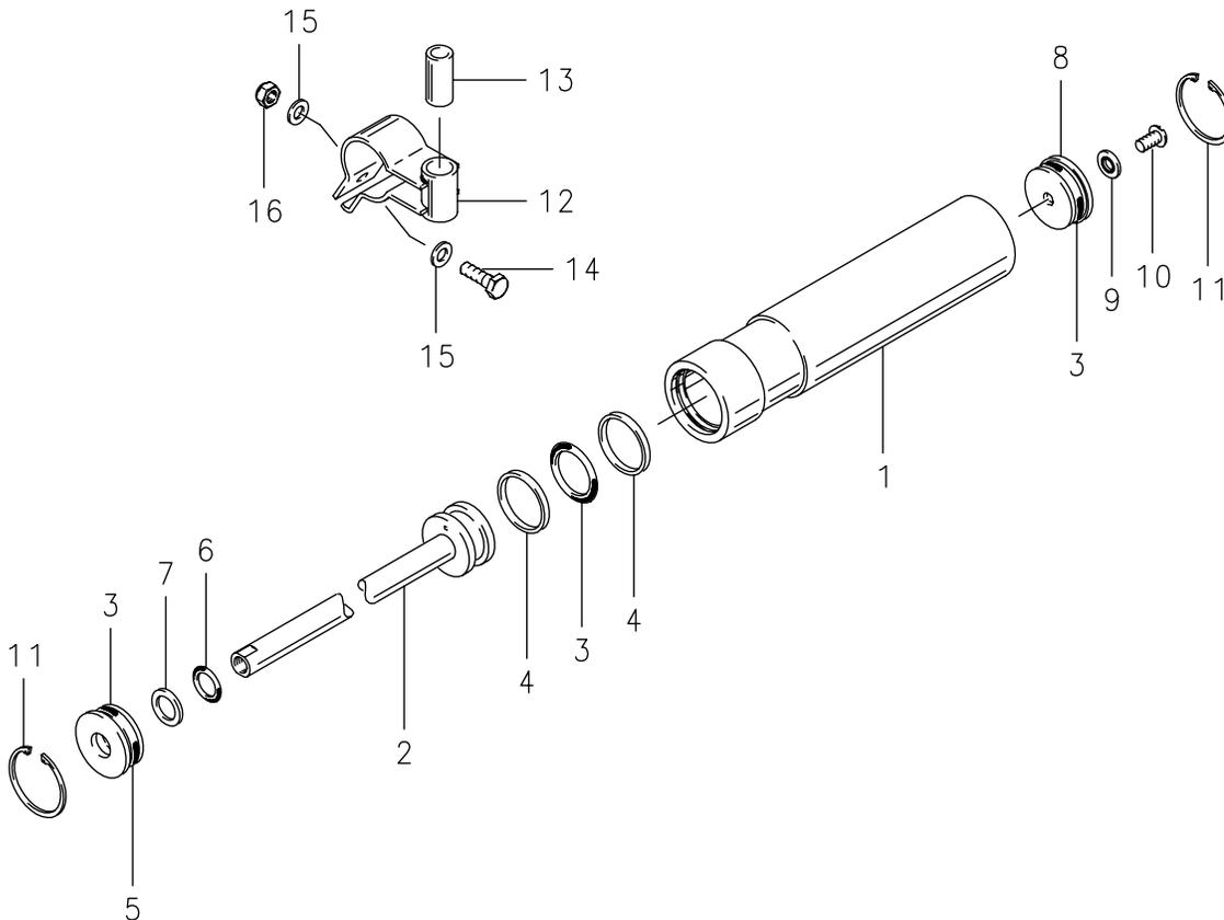
Note: Parts list for reference only. Contact airframe manufacturer to order shimmy dampers and components listed.
